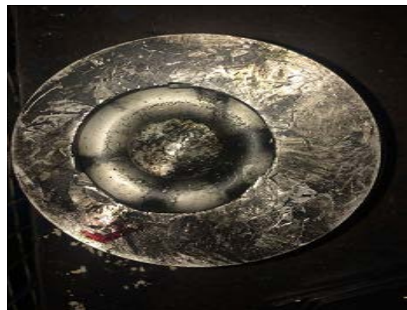
Figure 1a: Damaged piston
