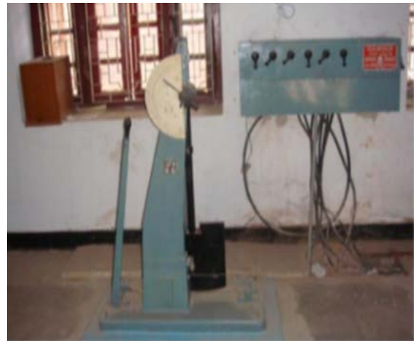
Figure 2.1: Charpy impact tester for toughness
