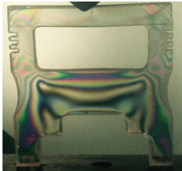
Fig 6: Fringes at load 104.3784N for Model-2
