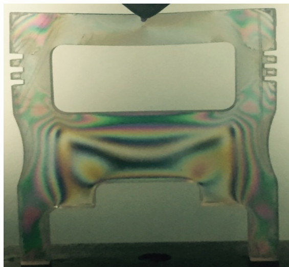
Fig 5: Fringes at load 104.3784N for Mode-1
