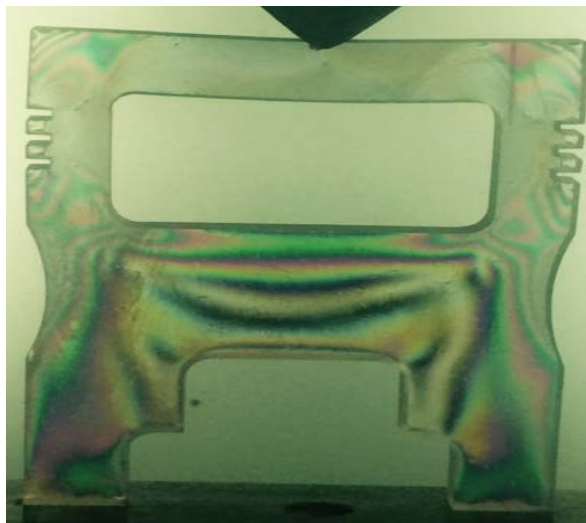
Fig 7: Fringes at load 104.3784N Model-3
