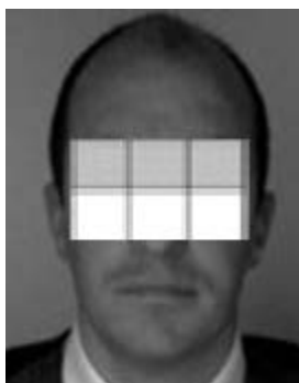
Figure 5: This SSR Filter shows that the Eye area is relatively darker than cheekbone area.
